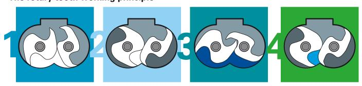
Atmospheric air is drawn through the inlet port into the compressor chamber as a result of the rotational action of the tooth rotors.
