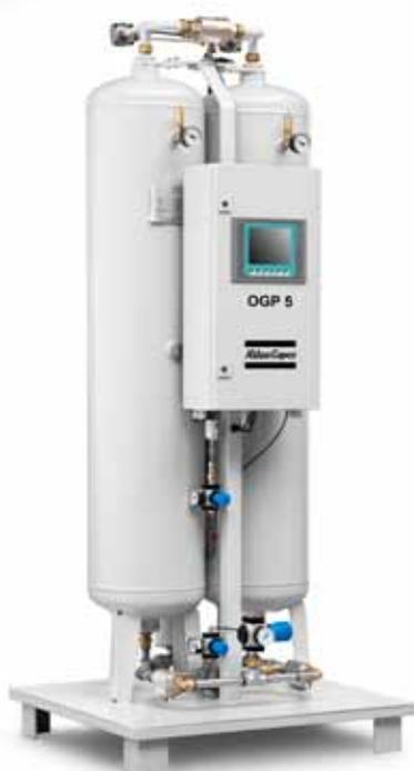
Atlas Copco's new oxygen generator uses Pressure Swing Adsorption technology to isolate oxygen molecules from other molecules in compressed air. The result is high purity oxygen at the outlet of the generator. The OGP series is a very cost-efficient source of oxygen used in various industries like waste water treatment, ozone production, health care, glass industry, and many others.
