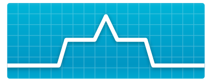
8% of all installations Factory working 2 shifts/day, no weekend work: typical 'fixed' speed application
