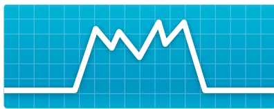
64% of all installations Factory working 24 hrs/day: low demand at night & high demand during the day
